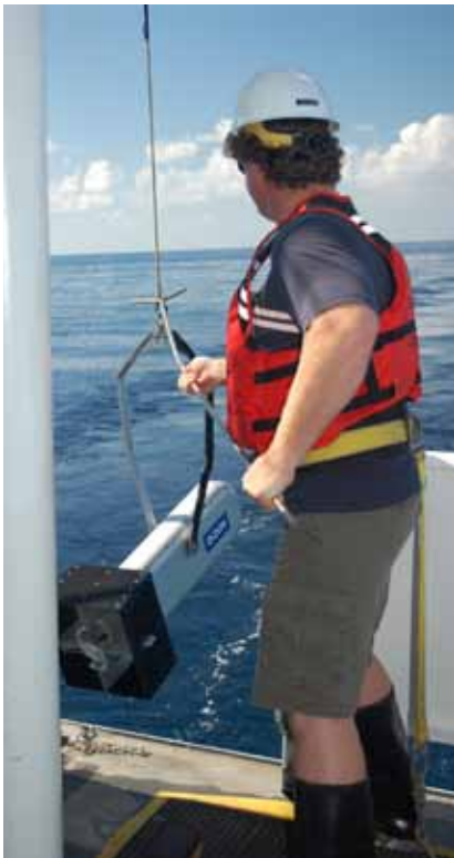
Survey Technician Frankie Daniel retrieves the Moving Vessel Profiler. Image courtesy NOAA. http://www.noaa.gov/features/04_resources/images/tj6.jpg
