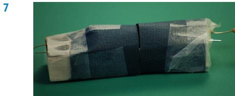
7. Repeat Step 6 to place a dome over the photocell. Leave a very small gap between the two pieces of construction paper that is just wide enough to slip the filter between the photocell and the LED.
