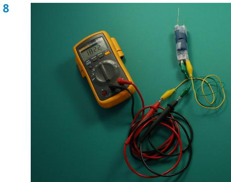
8. Using jumper cables, connect the multimeter leads to the two leads of the photocell, and set the meter to read resistance (ohms; abbreviated  $\Omega$ ). It does not matter how you connect the leads, as long as each of the two multimeter leads are connected to one of the photocell leads.
