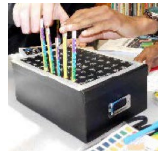
Figure 1. Image of seafloor box with sounding rods demonstrating the taking depth measurements.
