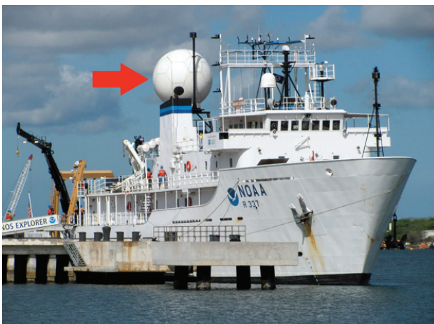
Telepresence: real-time, broadband video and audio communications made possible by the Okeanos Explorer 's powerful satellite antenna (red arrow).
