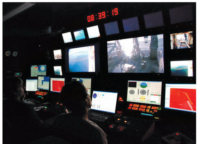
Arrays of monitors in the ship's control room and onshore in Exploration Command Centers display high-resolution streaming video of the remotely operated vehicle as it operates on the seafloor.
