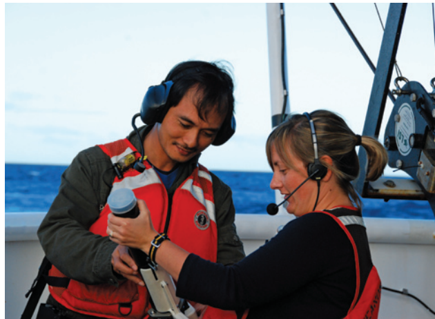
Scientists conduct an XBT cast which measures temperature through the water column.
