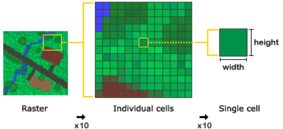
▲ Rasters are pixelated and made up with individual cells. The resolution of a raster is the height and width of that particular cell. In the case of bathymetry data, each cell would contain the depth of the seafloor within that area. Images adapted from ESR
