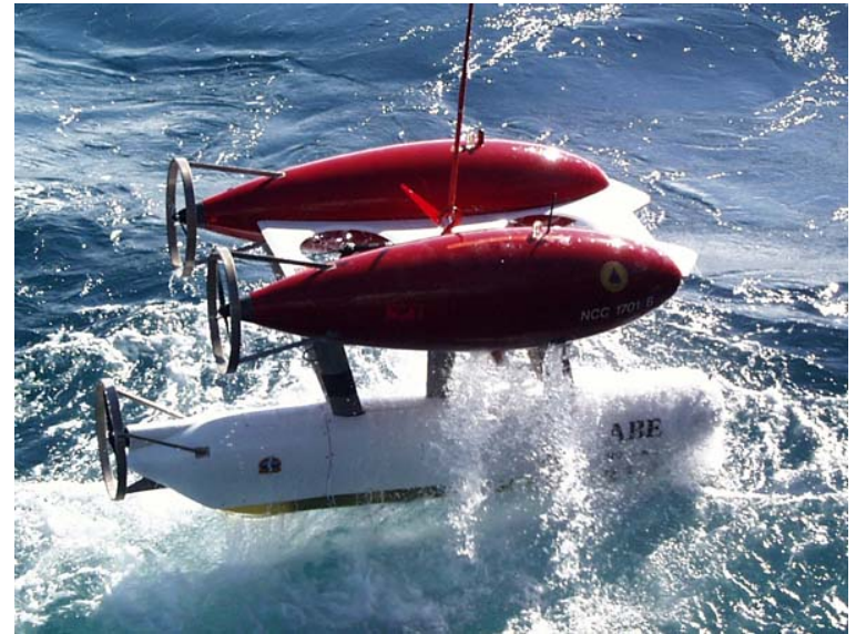
WHOI's Autonomous Underwater Vehicle, the Autonomous Benthic Explorer (ABE) being deployed. Photo: WHOI
