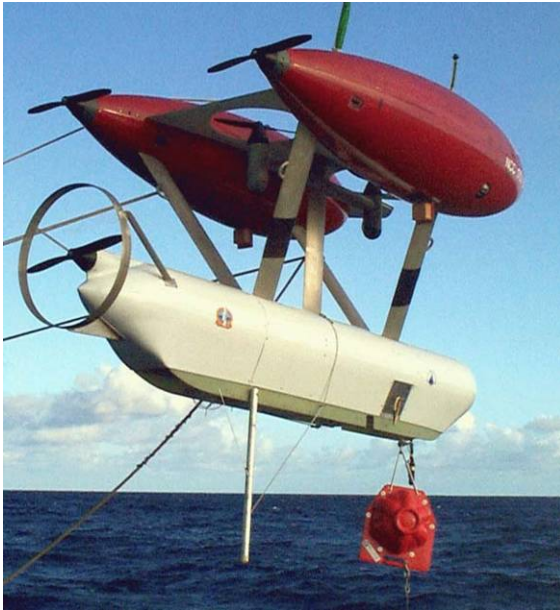
ABE's primary data collection tools are housed in the lowest of its three torpedo shaped pods, which is sealed. The two upper pods are free flooded and contain glass flotation balls. Photo: WHOI
