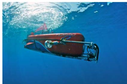
also acts as a backup for ascent and descent if the tilt mechanism for the horizontal thruster gets jammed due to coral rubble or other material getting caught in the caterpillar track that rotates them. PICASSO has one vertical tail fin and two fins for stability, and a maximum cruising speed of 1.6 knots. The vehicle is able to deploy either an HDTV camera or an autonomous visual plankton recorder in its main payload space.
