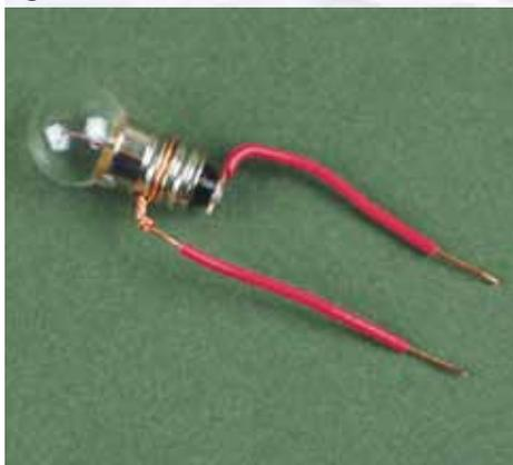
3. Cut two 3-inch lengths of insulated solid copper wire, and remove about 1/2-inch of the insulation from each end. These wires will be used as jumpers to make circuits by connecting sets of holes on the prototyping board.
